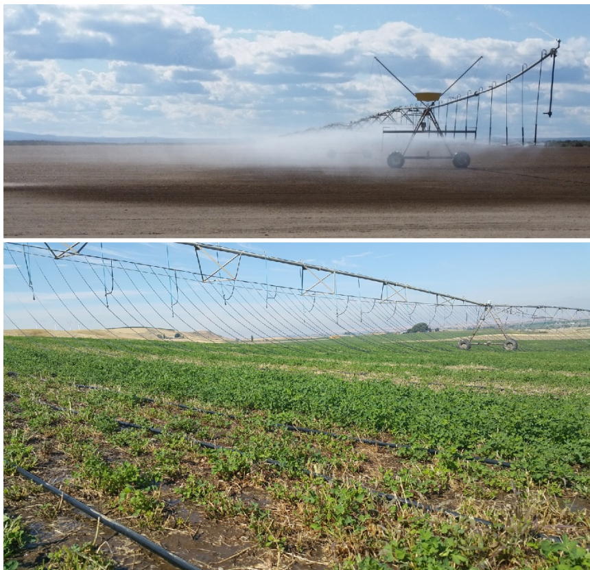
Figure 3-6. Center Pivot Sprinkler System (top) and Center Pivot System fitted with Mobile Drip Irrigation in an Alfalfa Field (bottom)
