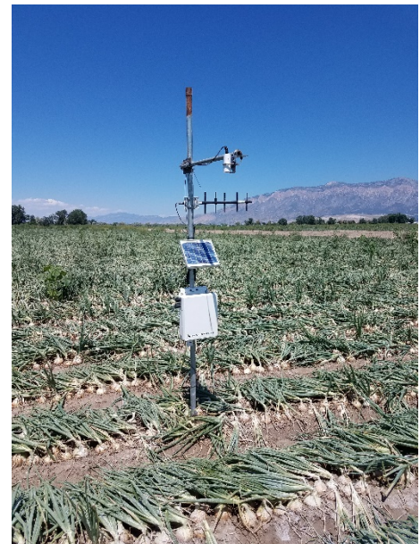
Figure 3-7. Soil moisture balance station; evaluating depletion accounting methods in Weber County, Utah
